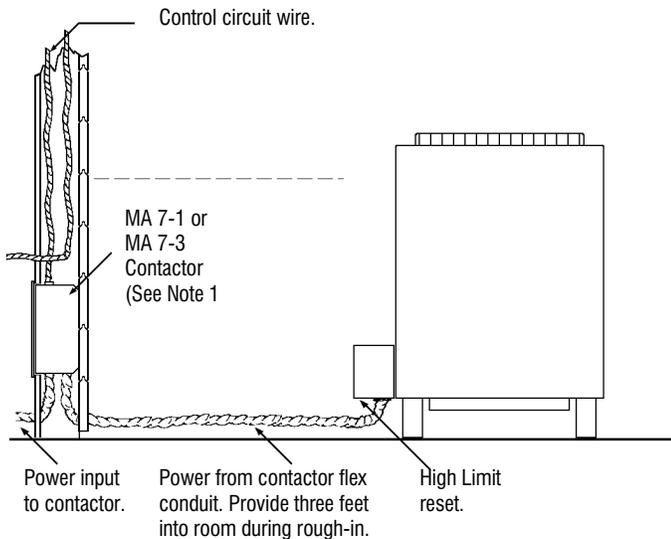
**Note 1:** The contactor box may be mounted anywhere outside the sauna room. A location should be selected so the front cover is accessible for service and the noise of the contactor pulling in will not be a nuisance.
